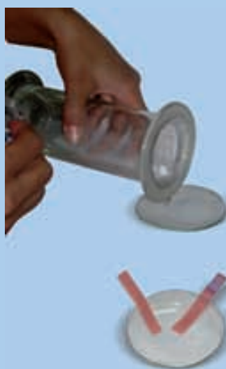
Fig. 4.4 (b) : Testing of solution with litmus papers
